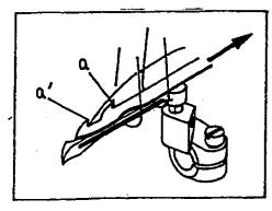
THE TRIMMING ABILITY OF KNIFE MUST BE MODERATE OR THE KNIFE WILL BE WORE OUT VERY SOON. IF THE TENSION OF KNIFE PRESSURE SPRING IS TOO BIG. YOU CAN ADJUST IT BY MOVING KNIFE PRESSURE SPRING TO THE RIGHT OR LEFT IN ORDER TO GET PROPER TENSION.
